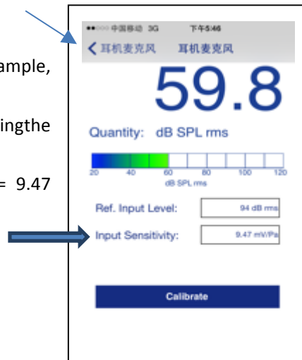
Fig 7. Sensitivity of the each i436 in User’s Manual
