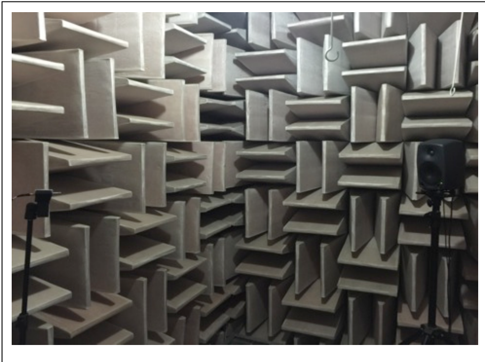
Fig. 5 Measurement setup for testing the frequency response
